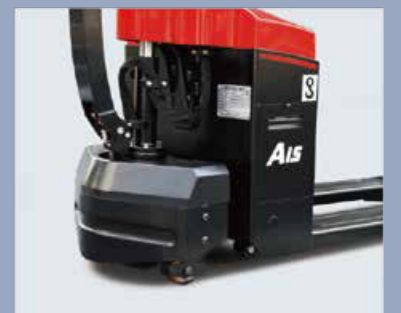
Auxillary wheels are equipped to have better stability
