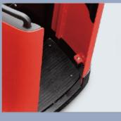
he pedal applies shock absorption esign, greatly improve the operator's omfort, reduce the fatigue
